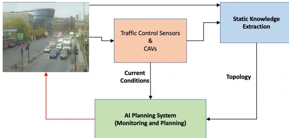
Figure 1. An overview of the proposed architecture for using AI Planning in Urban Traffic Control Extended with CAVs
